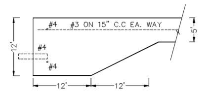
Note: Welded wire mesh shall only be permitted in sidewalk construction. The addition of poly mesh is acceptable in lieu of other sidewalk reinforcement.
