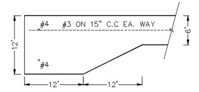
Where driveway meets garage slab, install 24" #4 dowels, with plastic sleeve on one end of dowel, on 24" centers and additional #4 bars top and bottom of beam.
